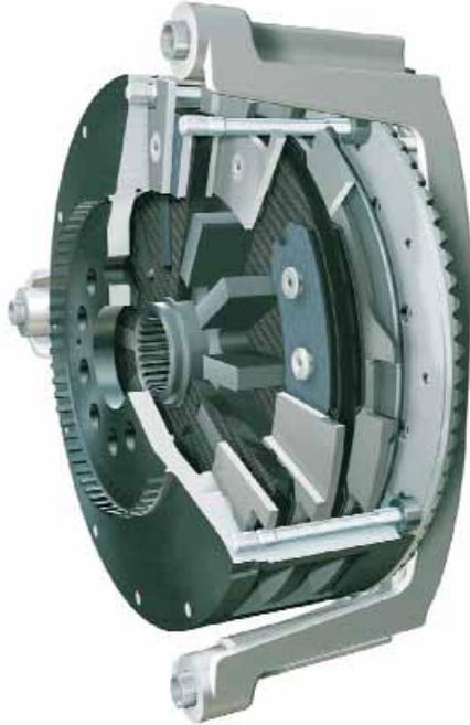
As has been mentioned above, a low center of gravity is very important for the competitiveness of a car. The engine of the Carrera GT in combination with a multi-disc clutch adopted from motorsport is ideally suited for a particularly low installation. The clutch disks are made of industrial ceramics similar to those used for the brake disks. This allows the required performance density to be realized without impairing the durability
