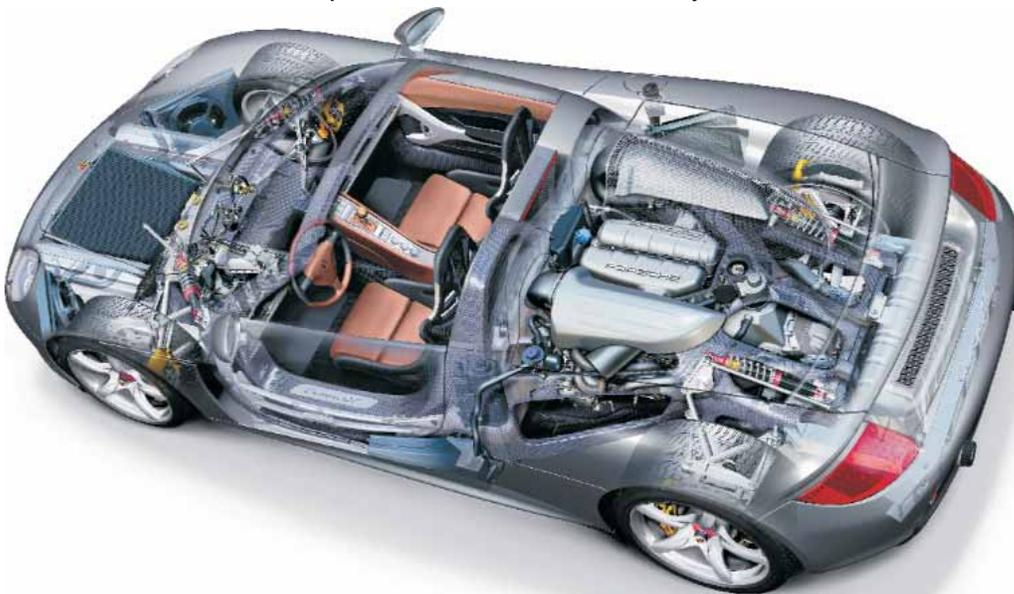
The entirely new "supporting structure" made of CRFP allowed significant progress to be made in terms of car weight and stiffness. Comprehensive mathematical analysis and optimizations were carried out taking into account the loads occurring during car operation and collisions. The highly integrated structure created for the Carrera GT stands out
